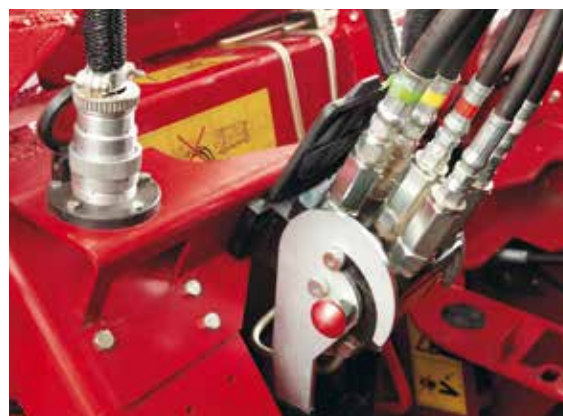
Mount the header in a matter of minutes with the single latch that connects all hydraulic functions
