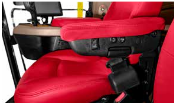
Air suspended seat or ventilated, heated, semiactive leather seat with controls to provide luxury automotive comfort level
