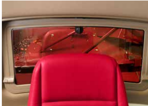
Large inspection window behind operator's seat
