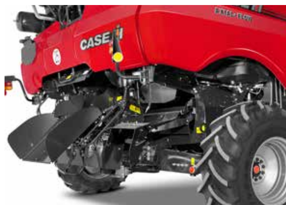
Straw spreader with different spreading options with spread widths up to 14 m
