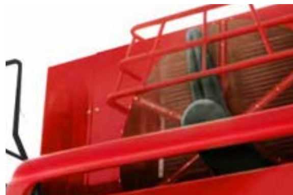
Fixed radiator grille for optimal dust clearing
