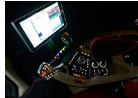
The icons on all switches are backlit when the headlights are on.
